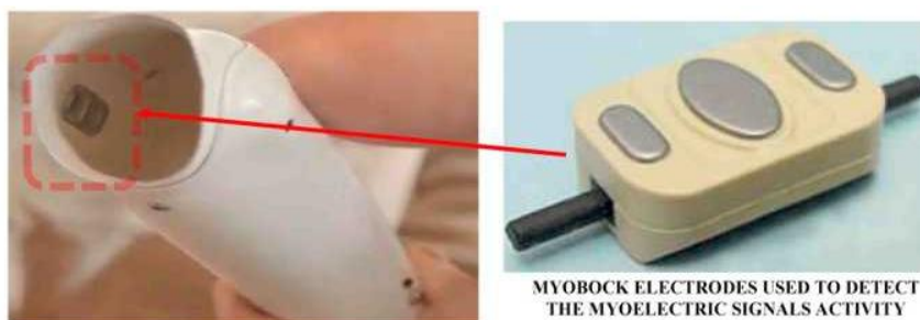
Figure 4. Myoelectrodes (MyoBock) from Ottobock installed in the prosthesis sleeve [10]
