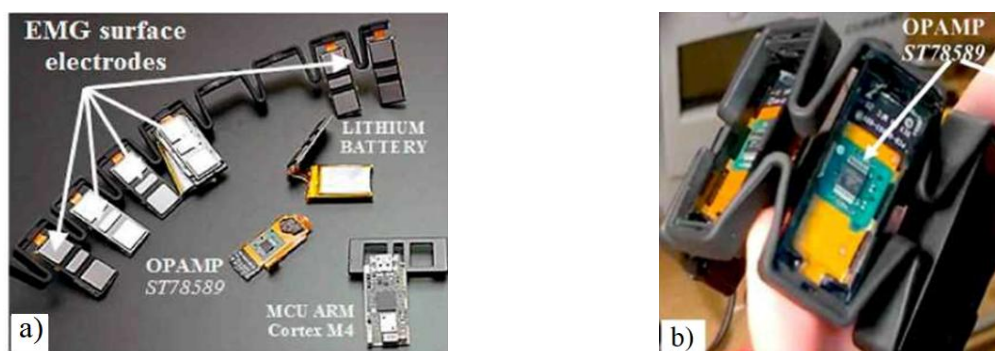
Figure 8. Myo Armband structure (a) and one electrode structure (b) [10]
